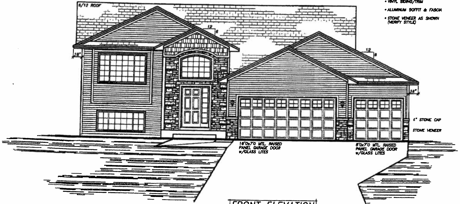
FRONT ELEVATION 1/4"=1'-0" 1220 SQ.FT. MAIN LEVELS
